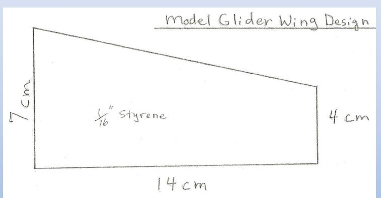
In the bottom of your kit box is a polystyrene sheet to make wings and rudders. Heavy duty scissors such as medical trauma scissors work well for cutting styrene. A utility knife may also be used. Remember to wear safety glasses or goggles.
